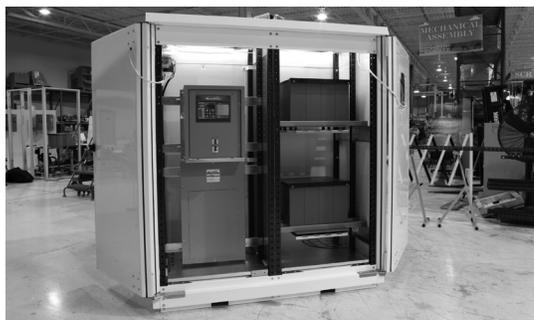
Figure 2e: Example of battery charger in NEMA 1 enclosure during production before wiring has been completed
